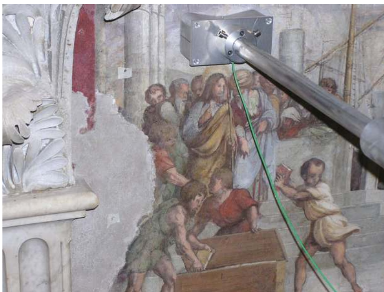
Figure 3. Single-sided NMR measuring moisture in a wall painting dating back to the XV century located in Nostra Signora del Sacro Cuore Church, Rome, Italy.
