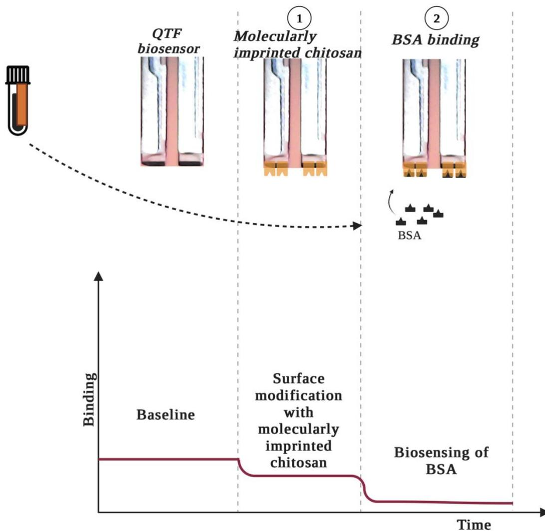
**Figure 2.** Schematic representation of biosensing of BSA with molecularly imprinted chitosan modified QTF-based sensor.
