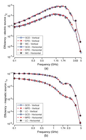
Fig. 5. Efficiency was evaluated with the realistic pectoral model for an (a) electric  $\eta_E$  and (b) magnetic  $\eta_H$  receiver implanted in the heart. Different receiver orientations (vertical and horizontal) and configurations {Surface Current Distribution (SCD), Electric (EPD) and Magnetic Point Dipole (MPD), out-of-plane Magnetic Current (MC) and Line Current (LC)} are compared.
