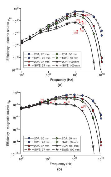
Fig. 3. WPT efficiency for (a) an electric  $\eta_E$  and (b) magnetic  $\eta_H$  receiver as a function of the frequency and the phantom radius  $R_p$  (asymptotically equivalent to the implantation depth) evaluated through the 2D-Axisymmetric (2DA) and the Spherical Wave Expansion (SWE) models. The red dots indicate the efficiency of physically realized WPT systems proposed in the literature and detailed in Table I.
