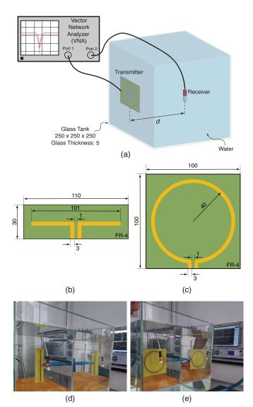
Fig. 2. Experimental evaluation of WPT efficiency in lossy media: (a) the transmitter is positioned outside a cubic glass tank filled with water, whereas the receiver designed in [44] is inside the tank at a distance d from the transmitter. Then, the scattering parameters are measured with a two-port VNA considering (b–d) an electric (dipole antenna), and (c–e) a magnetic (loop antenna) transmitter. All dimensions are in millimeters.
