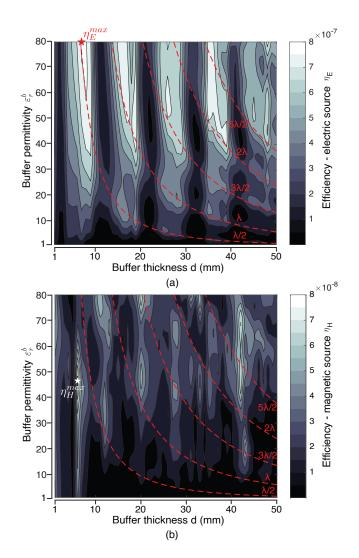
Fig. 7. Contour plots for the efficiency as a function of the buffer thickness d and permittivity  $\varepsilon_r^b$  for an (a) electric source  $\eta_E$  and a (b) magnetic source  $\eta_H$ . The star indicated the global maximum position, and the dotted lines indicate the position corresponding to  $\lambda/2$  its integer multiples as a function of  $\varepsilon_r^b$ .
