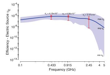
Fig. 8. WPT efficiency considering an optimal electric transmitter. The continuous blue line is the efficiency averaged (avg  $\eta_E$ ) over the 200 pacemaker positions. Besides, the blue area represents the maximum (max  $\eta_E$ ) and minimum (min  $\eta_E$ ) efficiency values. Finally, the red bars show the standard deviation on the efficiency  $\sigma_{\eta}$  at the ISM frequencies of 433 MHz, 915 MHz, and 2.45 GHz.
